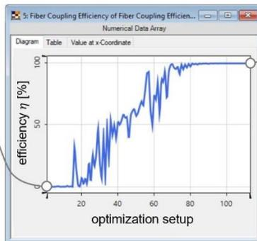
parametric optimization of coupling efficiency with downhill simplex algorithm
